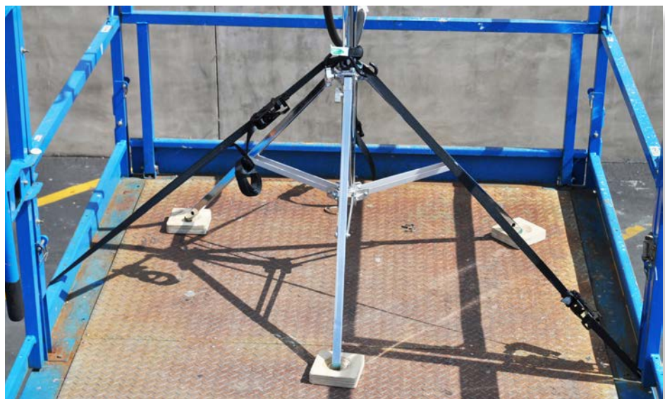
Figure 5.1. A lamp stand secured to a scissor lift platform with ratchet straps.
