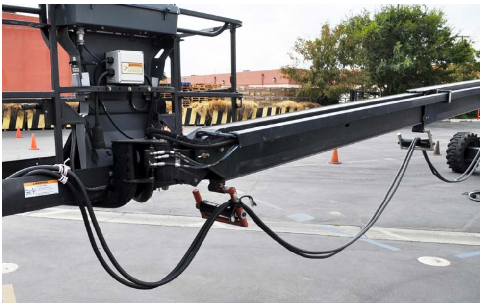
Figure 4.3. Electrical cables on cable rollers. The cable is tied to the first roller to allow for any horizontal or vertical movement of the platform.
