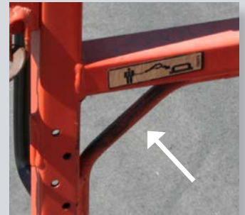
Figure 1.2. Anchor points are for fall protection use only. Do not attach equipment to an anchor point.
