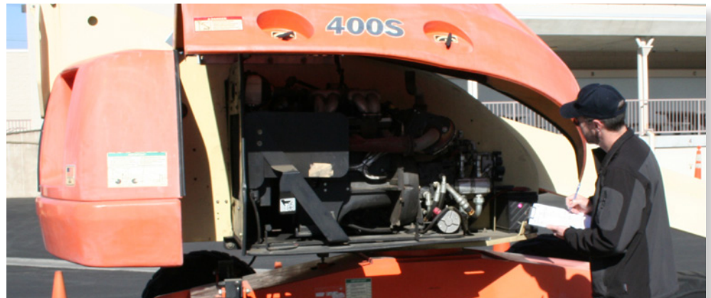
Figure 1.1. A walk-around inspection is required for boom lifts and scissor lifts.
