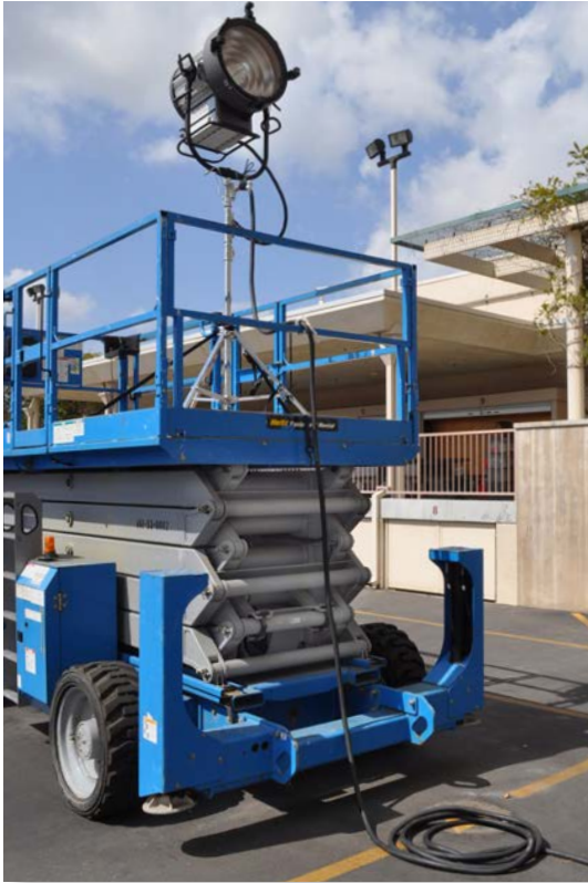
Figure 5.2. Secure cable to the guardrails of the platform (above) and run it down the narrow end of the scissor lift (left). Be sure there is enough cable to allow for raising the platform.
