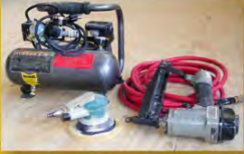
Air compressor and attachments.
