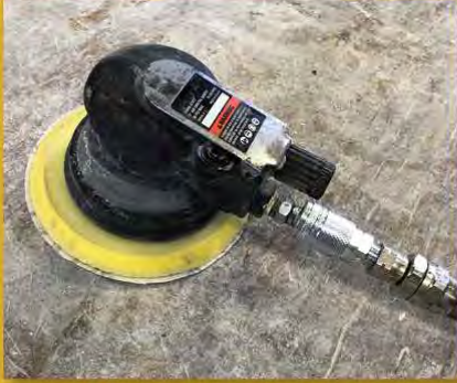
Power tools such as this pneumatic sander may create noise that is above safe levels for workers without hearing protection.
