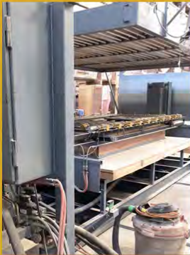
Molding plastic in a vacuum forming machine may produce hazardous gases or vapors.
