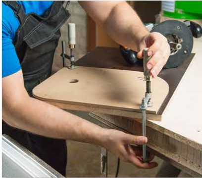
Clamp down a workpiece to keep it (or the tool) from kicking back.
