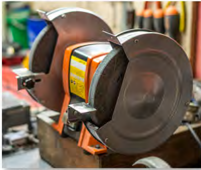
The space between the work rest and the grinding wheel must not be more than 1/8 of an inch.
