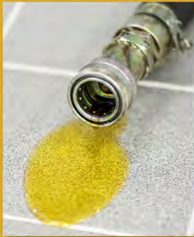
Spilled or leaking hydraulic fluid can create a slippery work surface.
