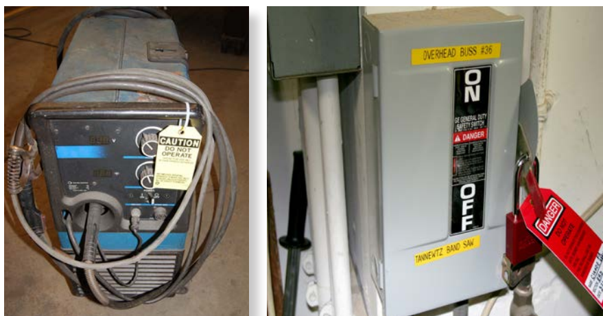
Figure 2.11. Disconnect (left) or de-energize (right) equipment before performing any installation, maintenance, or repair.
