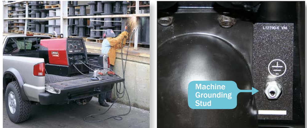
Figure 2.7. When on a vehicle, the welder must be properly bonded (left) using the machine grounding stud (right).
