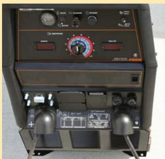
Figure 2.8. Cord-and-plug connected welders must be grounded using a 3-plug electrical outlet.
