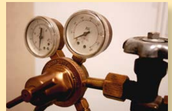
Figure 1.10. Keep regulators and connectors clean and free of oil or grease.
