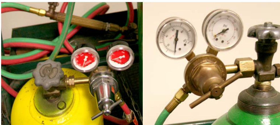
Figure 1.8. Regulators and gauges are gas specific and are not interchangeable.
