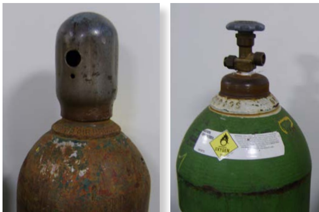
Figure 1.5. Valve cap (left) and no valve cap (right).
