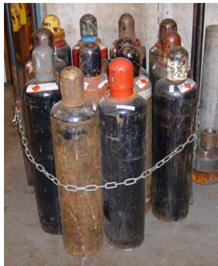
Figure 1.4. Cylinders must be strapped or chained to protect against tipping or movement.
