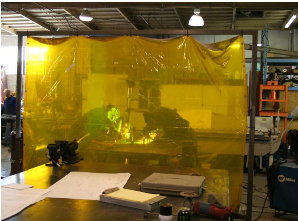
Figure 6.5. Welding area isolated by a tinted curtain, designed to absorb welding rays.
