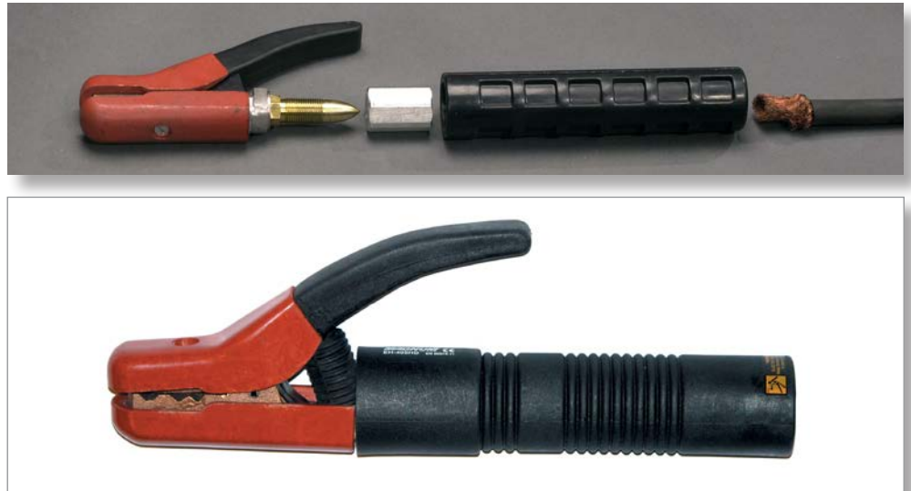
Figure 2.9. An electrode holder in exploded view (top) and ready for use (bottom).
