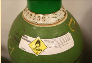
Figure 1.2. All cylinders must be legibly marked with the contents.
