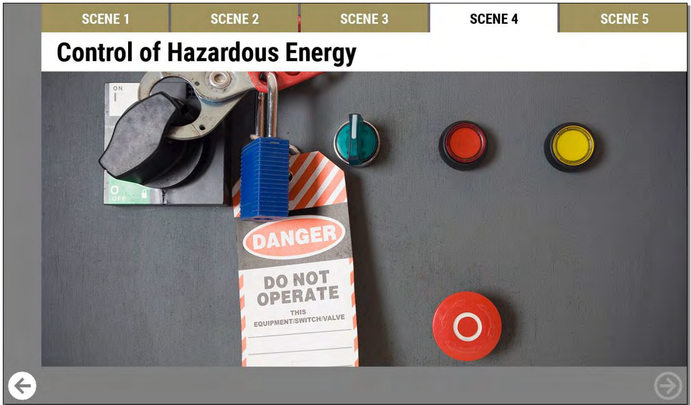
Scene Four, Control of Hazardous Energy.
